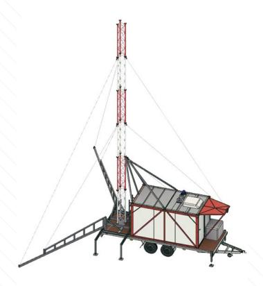
**Cell on Wheels (COW) Strommontazh** is designed to accommodate and operate the equipment of a cellular base station, exclude unauthorized access to the equipment and maintain the required temperature inside. COW is used to increase the capacity of a cellular network or create a coverage area due to a sharply increasing load in a local region for a limited period. The permanent presence of personnel for operation is optional.
